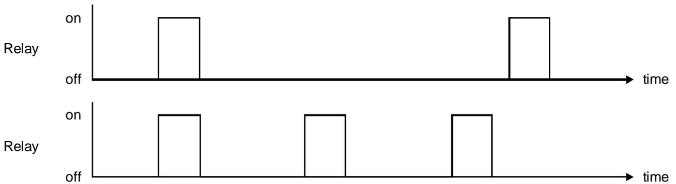
In frequency modulation mode the relay on time is fixed. A minimum relay off time can also be set. The control program will vary the actual off time to suit the error seen between the setpoint and the measured value at the time. For example if extra input is needed to reach the setpoint then the off time will be reduced resulting in more on pulses per period of time i.e. the frequency of the pulses is controlled to allow the setpoint to be maintained.
