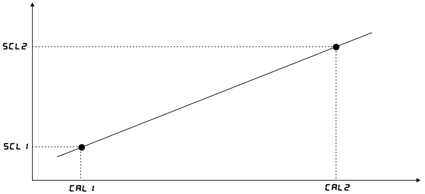
Two scaling points - display is linear
