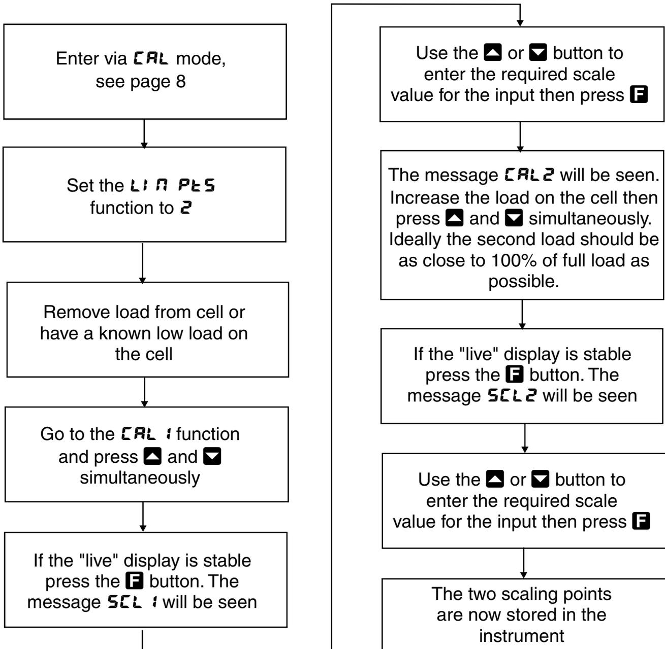
Note: If the "live" display at any scaling point is not stable then check the input signal for stability.
