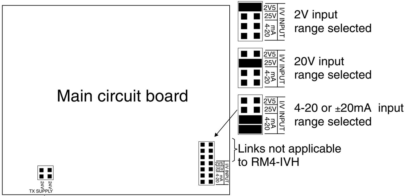
24V transmitter supply (20mA max.) links. Both links must be in for 24V supply.
