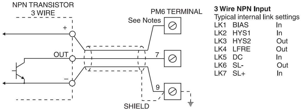
Notes: Use terminal 5 for 24V (20mA max) or terminal 11 for 5V (20mA max) or use external excitation. The LFRE link (LK4) when **In** can be used to help filter out high frequency noise and contact bounce provided that the maximum input frequency of the pulse signal is less than 80Hz.
