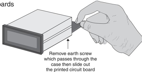
4. Configure the PCB links as required, see appropriate chapter
