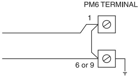
**Remote inputs for totaliser reset etc.**
