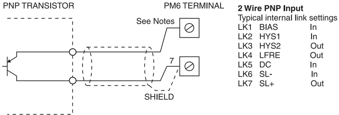
Notes: Use terminal 5 for 24V (20mA max) or terminal 11 for 5V (20mA max) or use external excitation. The LFRE link (LK4) when **In** can be used to help filter out high frequency noise and contact bounce provided that the maximum input frequency of the pulse signal is less than 80Hz.
