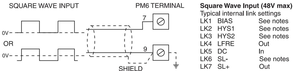
Notes: Inputs 100mV to 2.5V HYS2 (LK3) is **In**, HYS1 (LK2) is **Out**. Inputs above 2.5V HYS2 is **Out**, HYS1 is **In**. For inputs above 24V SL- (LK6) is **Out**. BIAS link (LK1) should be **In** if the signal does not go below 0V. The LFRE link (LK4) when **In** can be used to help filter out high frequency noise and contact bounce provided that the maximum input frequency of the pulse signal is less than 80Hz.
