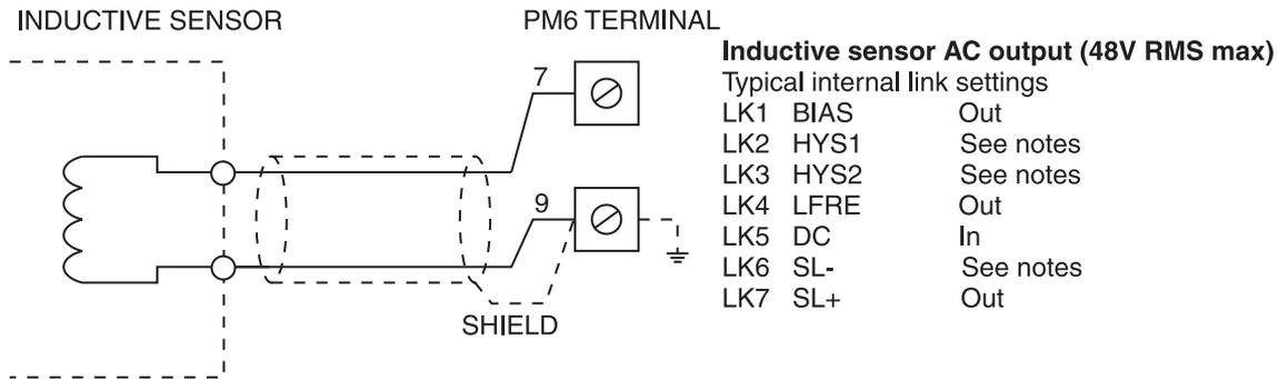
Notes: Inputs 100mV to 2.5V HYS2 (LK3) is **In**, HYS1 (LK2) is **Out**. Inputs above 2.5V HYS2 is **Out**, HYS1 is **In**. For inputs above 24V RMS SL- (LK6) is **Out**. The LFRE link (LK4) when **In** can be used to help filter out high frequency noise and contact bounce provided that the maximum input frequency of the pulse signal is less than 80Hz.
