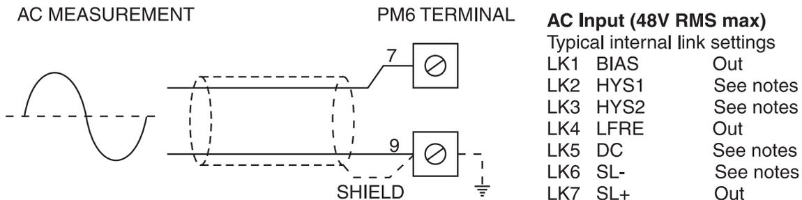
Notes: Inputs 100mV to 2.5V HYS2 is **In**, HYS1 is **Out**. Inputs above 2.5V HYS2 is **Out**, HYS1 is **In**. For inputs above 24V RMS SL- is **Out**. DC link LK5 should be **In** if the frequency will not be greater than 10Hz. The LFRE link (LK4) when **In** can be used to help filter out high frequency noise and contact bounce provided that the maximum input frequency of the pulse signal is less than 80Hz.
