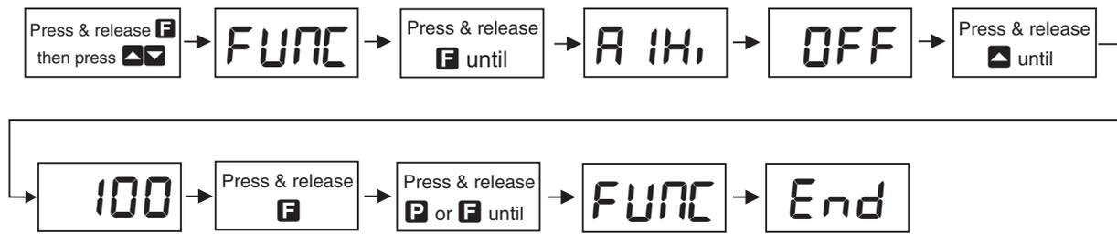
Example: Entering **CAL** mode to change decimal point function **dCPT** from **0** to **0.02**
