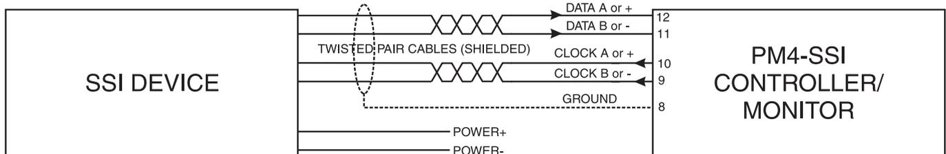
Maximum cable length: Maximum cable length is normally determined by the device being connected to the PM4. Consult the handbook for the SSI device used for details of maximum cable length. Notes: Twisted pair cable must be used for clock and data. refer to the **SSI F&E** function for details of clock frequency settings which may be required for long cable lengths and to the section on link settings below.
