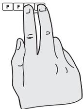
3. Within 2 seconds of releasing the **F** button press, then release the **▲** and **▼** buttons together. The display will now indicate **FUNC** followed by the first function.
