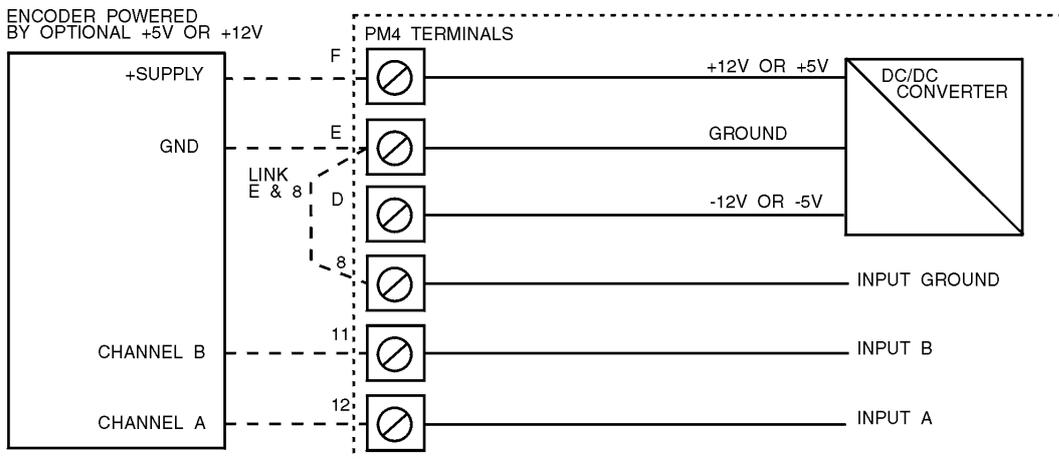
The optional supply can also be configured for 10V or 24V DC power supply and connected as shown below. It is necessary to link terminals D and 8 to couple the power supply and input grounds. The maximum current available is 20mA @ 24V and 40mA @10V.
