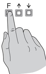
2. When the "wake up" messages have finished and the display has settled down to its normal reading press, then release the **F** button. Move to step 3 below.
