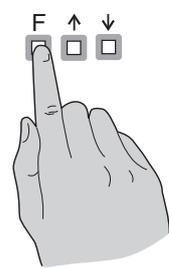
1. When the "wake up" messages have finished and the display has settled down to its normal reading press, then release the **F** button. Move to step 2 below.
