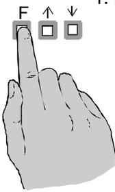
1. Remove power from the instrument and wait 5 seconds. Hold in the **F** button and reapply power. The display will indicate **CAL** as part of the "wake up messages" when the **CAL** message is seen you can release the button. Move to step 2 below.
