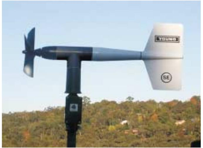
The Model WS-09101 Wind Monitor (the Wind Monitor-SE) combines the performance and durability of the standard Wind Monitor with a unique optical encoder wind direction transducer and serial output signal.
