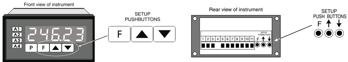
The instrument push button locations are shown above, some display types do not have front panel push buttons.
