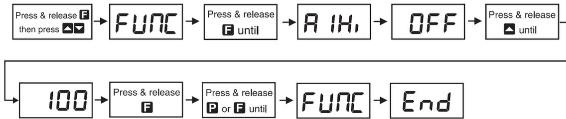
Example: Entering **CAL** mode to change decimal point **CH1 dCPT** function from **0** to **0.02**
