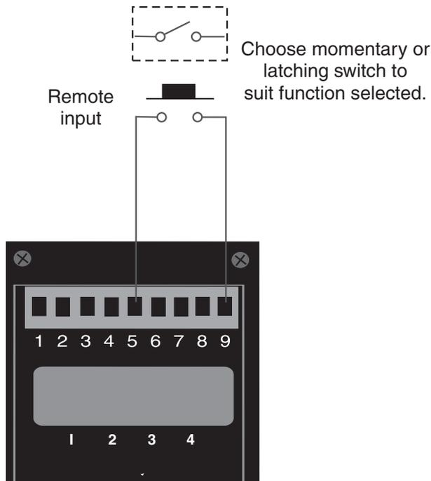
The selected remote input function can be operated via an external contact closure via a switch, relay or open collector transistor switch.
