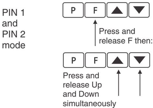
If a PIN has been set the message **Code** will be seen. Use **▲** or **▼** to enter the PIN then press **F** to accept the PIN.
