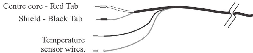
If dual temperature sensors are fitted then the colour code is:
