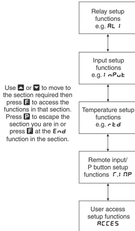
The example in the flowchart below shows the method using alarm relay 1 setup function (example only, actual functions seen may vary depending on software version).
