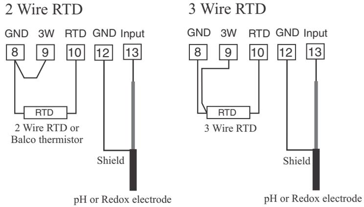
Termination of a typical pH electrode with temperature compensation for screw terminal connection
