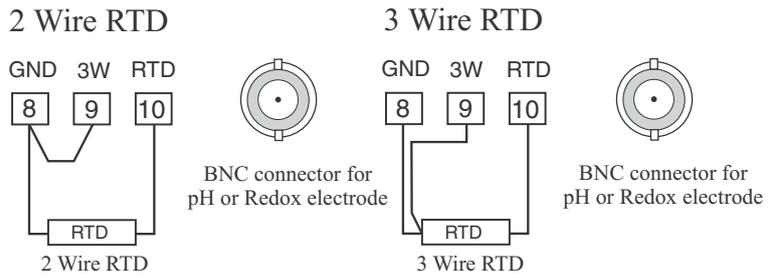
Rear sensor connection for panel meter without BNC connector (4 digit LED or 4 or 6 digit LCD display)
