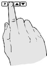
1. Remove power from the instrument. Hold in the **F** button and reapply power. The display will briefly indicate **CAL** as part of the "wake up messages" when the **CAL** message is seen you can release the button. Move to step 2 below.
