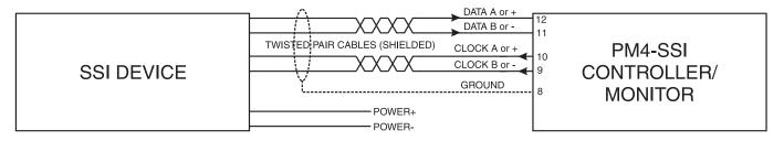
Maximum cable length: Maximum cable length is normally determined by the device being connected to the PM4. Consult the handbook for the SSI device used for details of maximum cable length. Notes: Twisted pair cable must be used for clock and data. refer to the **55**: FREE function for details of clock frequency settings which may be required for long cable lengths and to the section on link settings below.
