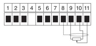
Note: Links LK7 & LK8 Must be set to SLIDE WIRE for Slide Wire input all other links should be out.
