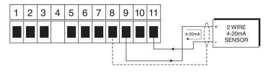
2 wire 4-20mA externally powered sensor
