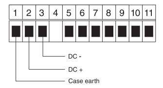
2 wire 4-20mA powered from non isolated regulated 18V supply (25mA maximum)
