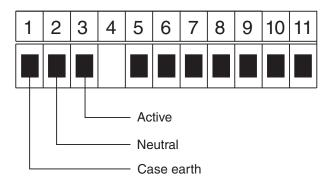
DC power connections (12 to 48VDC) - supply type is factory configured, check before connecting
