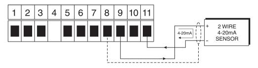
2 wire 4-20mA externally powered sensor
