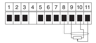
Note: Links LK7 & LK8 Must be set to SLIDE WIRE for Slide Wire input all other links should be out.
