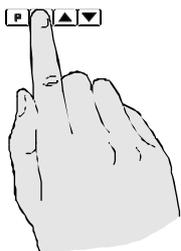
2. When the "wake up" messages have finished and the display has settled down to its normal reading press, then release the **F** button. Move to step 3 below.
