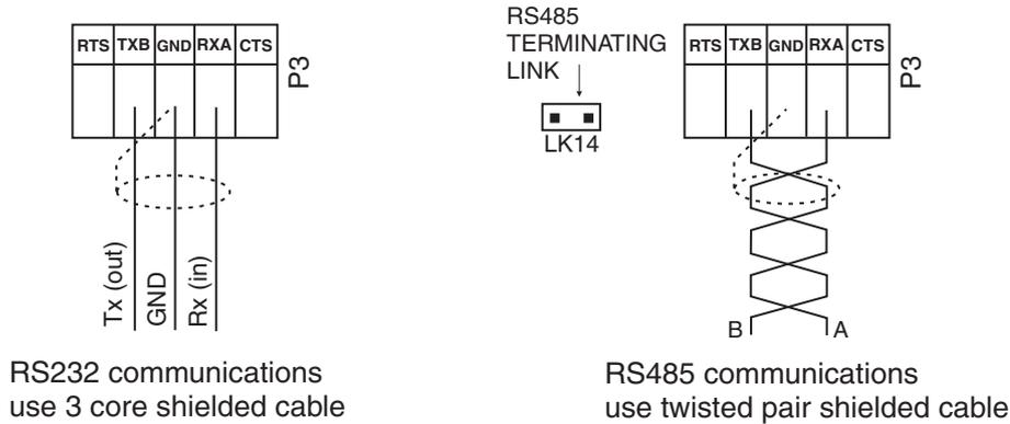
Notes: When connecting using RS232 in most cases the Tx line at the display connects to the Rx line at the device it is communicating with and the Rx line at the display connects to the Tx line at the other device, see diagram below.
