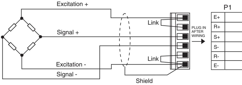
6 wire load cell/pressure sensor connection
