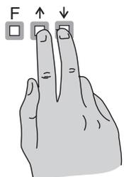
3. Within 2 seconds of releasing the **F** button press, then release the **▲** and **▼** buttons together. The display will now indicate **FUNC** followed by the first function.
