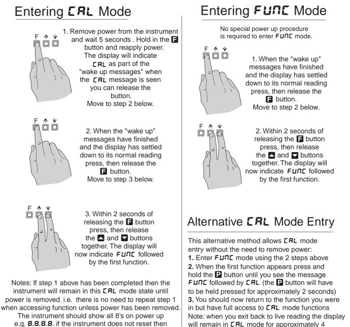
these numbers will not be seen. Switch off the instrument and allow a longer time delay before powering up again.
