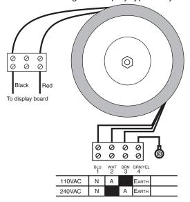
Low voltage AC supplies. For 100mm/200mm LED or 100mm electromagnetic display types only.
