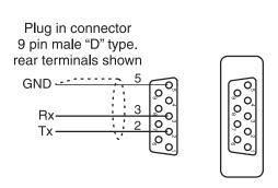
RS232 port for use in **A.b.** mode with Windows PC software purchased for use with this instrument or for on site software update only. This port will be disabled if the optional serial communications port fitted. If this port is to be used for **A.b.** communcation the **SEF. !LYPE** and **SEF. ?LYPE** functions must be set to **PDDE**
