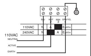
Important note: the 240V & 110V supplies use the same transformer, low voltage instruments use a different transformer. Do not use a low voltage transformer for 240V or 110V or vice versa.
