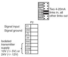
The supplies can be configured as 5, 10, 12 or 24V DC 25mA max. for 5, 12 or 24V 50mA max for 10V
