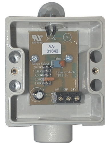
Model WS-TPVLL0 with 0-10VDC output with cover removed showing range selection jumpers.
