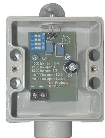
Model WS-TPLLO with 4-20mA output with cover removed showing range selection switches.
