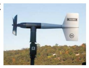
The Model WS-09101 Wind Monitor (the Wind Monitor-SE) combines the performance and durability of the standard Wind Monitor with a unique optical encoder wind direction transducer and serial output signal.
