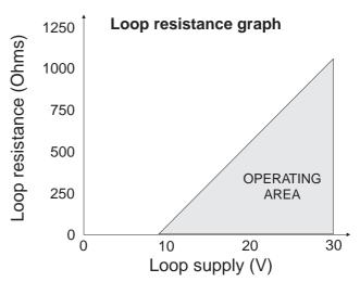
(Loop supply) - 9V Maximum loop resistance (Ohms) =
